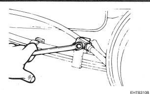
5. Remove the shackle assembly to separate the spring assembly from the frame.
