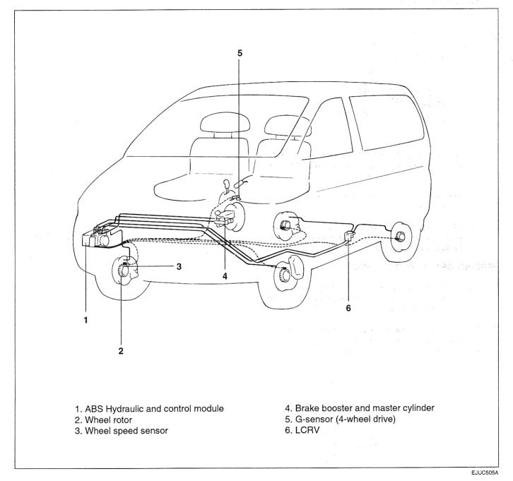
The Anti-Lock Brake System (ABS) controls the hydraulic brake pressure of all four wheels during braking on hazardous road surfaces, preventing the wheels from locking up. ABS provides the following benefits :
