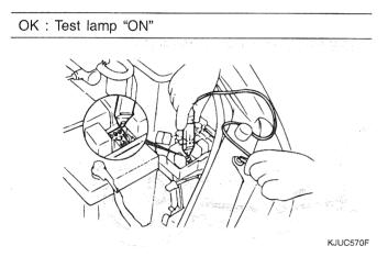
5. Apply the battery voltage to the terminal No.4
