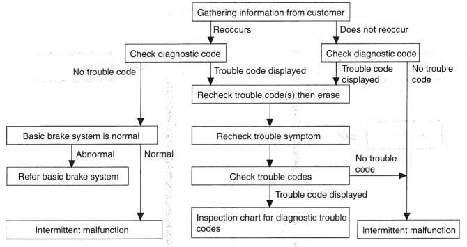
\* Using the customer problem analysis check sheet for reference, ask the customer as much detail as possible about the problem.
