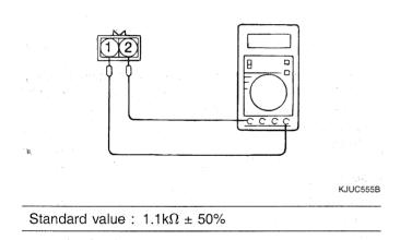
3. Check the speed sensor cable for breakage, damage or disconnection; replace with a new one if a problem is found.
