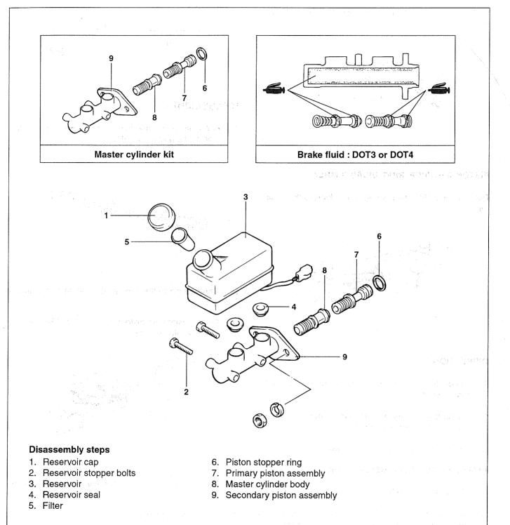
CAUTION Do not disassemble the primary and secondary piston assembly.
