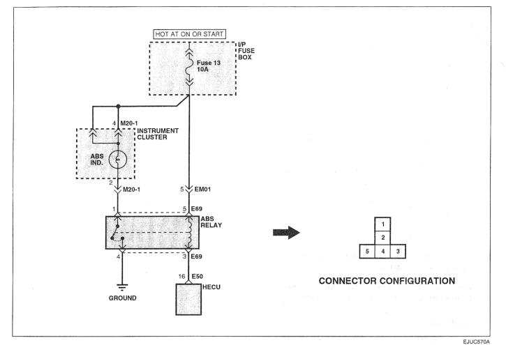
1. Turn the ignition switch OFF and disconnect the ABS relay from engine room relay box.
