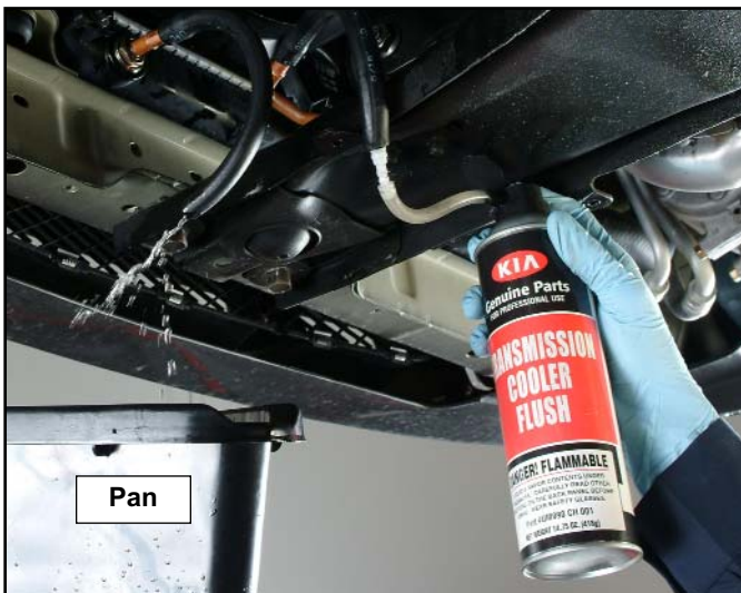
Flushing Through A/T Cooler Outlet Hose (Sephia/Spectra/Rio Shown)
