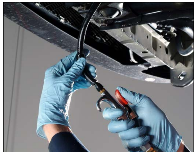
Drying A/T Cooler With Shop Air
