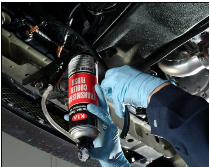
Invert Can to Clean Out Flush Fluid
