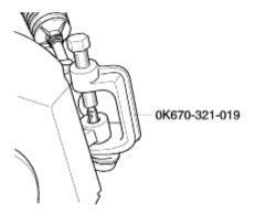
7.Remove lower arm cotter pin using a ball joint remover, and remove lower arm from steering knuckle.
