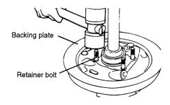
Apply gummed cloth tape around the edge of the bearing case for protection.
